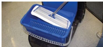
Place pre-moistened mop head (white side up) in bucket filled with recommended 150–200cc of water and chemical per mop. Press mop head against mop frame so the Velcro® system fastens.
